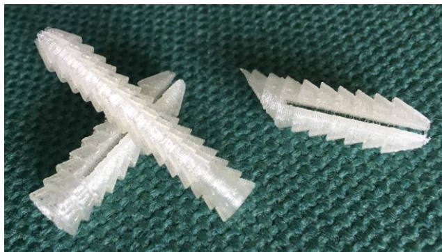
Figure 5: Different dowels printed from a parameterized 3D model [14]
